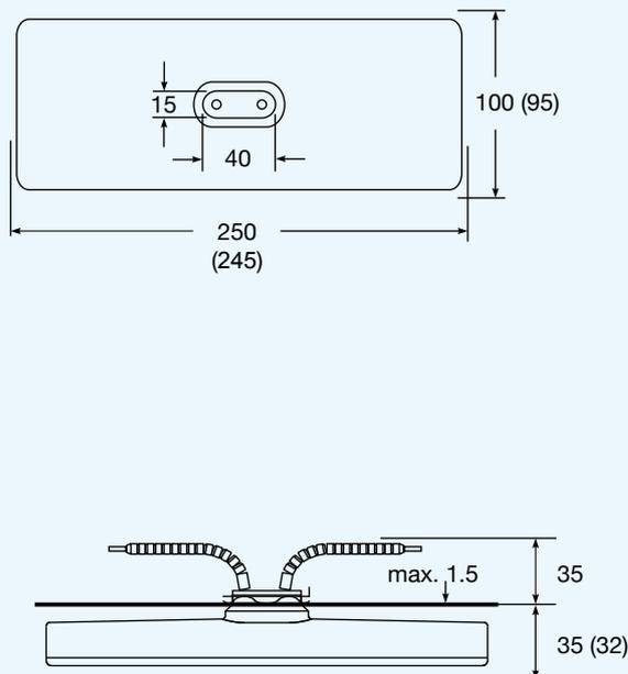
Figure 2: Mounting dimensions and radiator dimensions ( ) in mm
