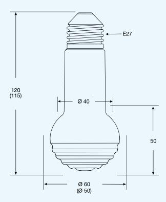
Figure 2: Mounting dimensions and radiator dimensions () in mm
