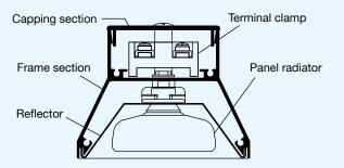
Fig. 77: Cross-section through an EBF construction element
