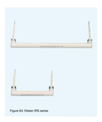
Elstein IRS rod radiators are ceramic infrared radiators, designed for operating temperatures of up to 650 °C. With the help of MPO and MPO/2 mounting profiles, surface ratings of up to 72.0 kW/m² can be realised.
