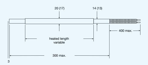
Figure 2: Mounting dimensions and radiator dimensions () in mm
