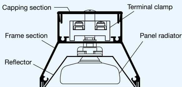
Fig. 77: Cross-section through an EBF construction element
